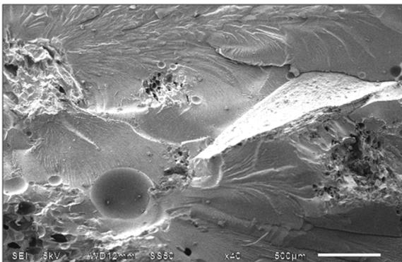
**Figure 5:** SEM for 15 wt% of bagasse fiber in epoxy resin at magnification 50X.
