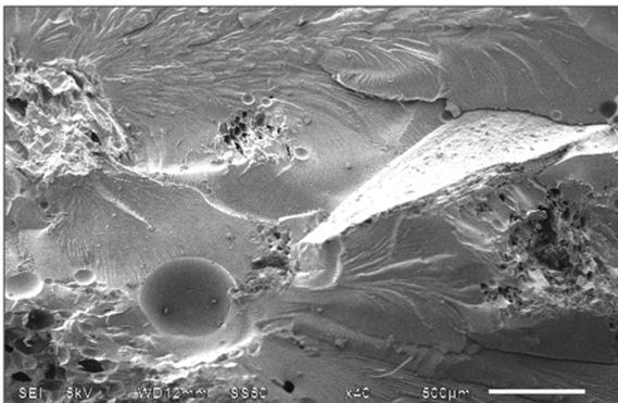
**Figure 4:** SEM for 10 wt% of bagasse fiber in epoxy resin at magnification 40X.
