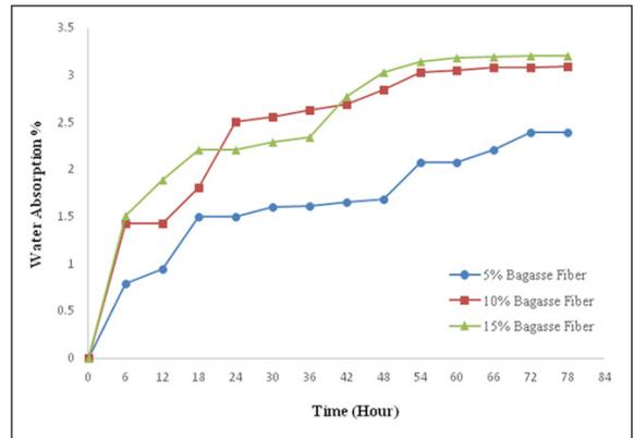
**Figure 2:** Effect of varying wt% of bagasse fiber on water absorption.
