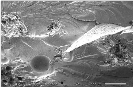
**Figure 3:** SEM for 5 wt% of bagasse fiber in epoxy resin at magnification 40X.
