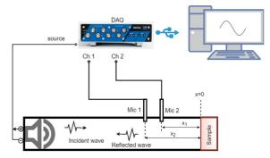
**Figure 1**: Schematics of SAC measuring set-up [5]. Reproduced from [5] with permission from Elsevier.
