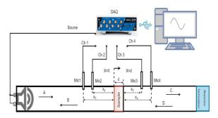
**Figure 2**: Schematics of STL measuring set-up [5]. Reproduced from [5] with permission from Elsevier.
