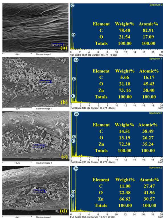
**Figure 6:** FE-SEM and EDS elemental analysis of (a) untreated cotton, coated cotton fabrics with Zn3 nanoparticles after repeated washing for various cycles (b) 10 washed, (c) 20 washed and (d) 30 washed.
