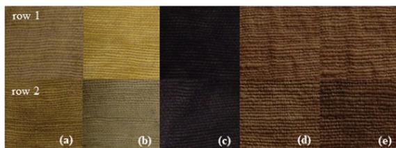
**Figure 8:** Color shade of uncoated cotton (row 1) and cotton coated with CZn4 nanoparticles (row 2) and dyed with *Terminalia catappa* Linn. powder for various mordants as (a) control, (b) Alum, (c) FeSO<sub>4</sub>, (d) Cu (II) SO<sub>4</sub>, and (e) Tannin.
