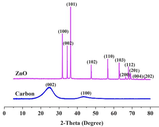
Figure 2: XRD patterns of ZnO and carbon nanoparticles.
