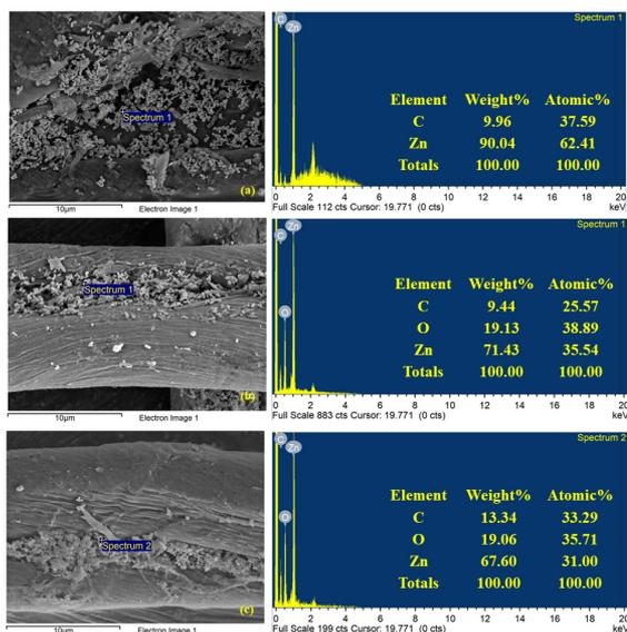
**Figure 7:** FE-SEM and EDS elemental analysis of CZn4 nanoparticles after repeated washing for various cycles (a) 10 washed, (b) 20 washed and (c) 30 washed.
