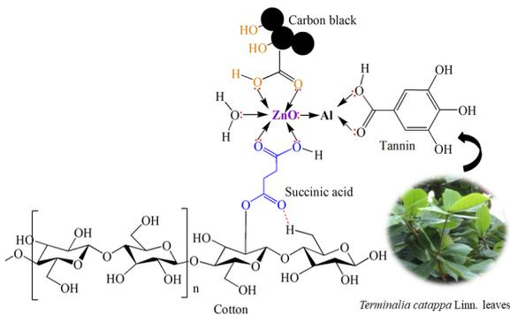
**Figure 1:** Proposed mechanism for the cotton fabric coated with ZnO and carbon black nanoparticles dyed with *Terminalia catappa* leaves powder.
