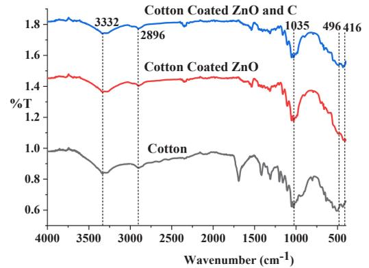
Figure 4: ATR-FT-IR spectra of uncoated cotton, cotton coated ZnO and carbon black nanoparticles.
