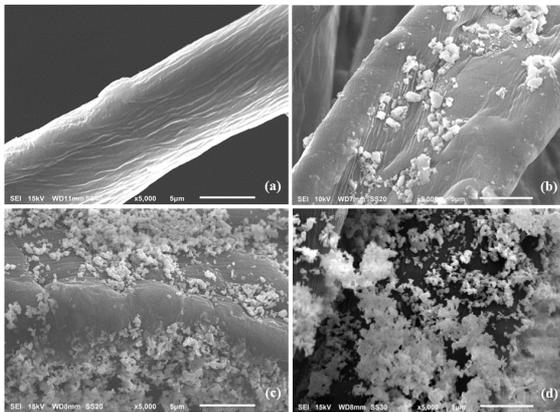
Figure 3: SEM images of (a) uncoated cotton, (b) cotton coated carbon, (c) cotton coated ZnO and (d) cotton coated CZn4 nanoparticles.
