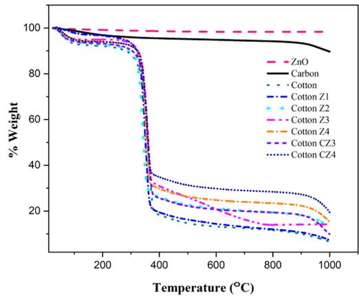
Figure 5: TGA curve of ZnO, carbon, uncoated cotton, cotton coated Z1, cotton coated Z2, cotton coated Z3, cotton coated Z4, cotton coated CZ3, and cotton coated CZ4.
