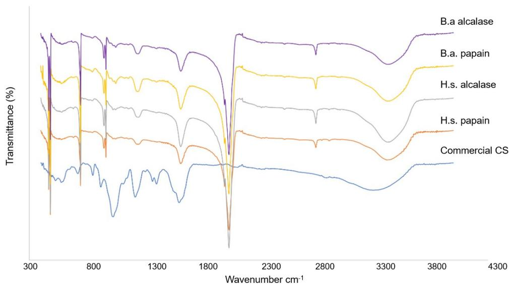
**Figure 4:** FTIR spectrum of commercial CS, standard bovine sodium chondroitin-4-sulphate; WSC papain, chondroitin sulfate from *Holothuria scabra* extraction by papain; WSC alcalase, chondroitin sulfate from *Holothuria scabra* extraction by alcalase TSC papain, chondroitin sulfate from *Bohadschia argus* extraction by papain; TSC alcalase, chondroitin sulfate form *Bohadschia argus* extraction by papain. T%, Transmittance.
