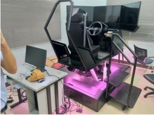
**Figure 3:** A six-degree-of-freedom motion base driving simulator.
