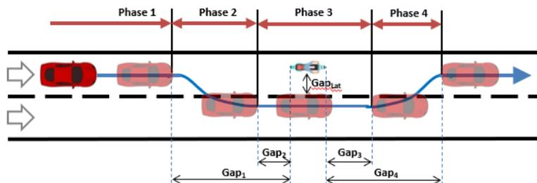
**Figure 2:** Four phases of the car-to-motorcycle overtaking maneuver.
