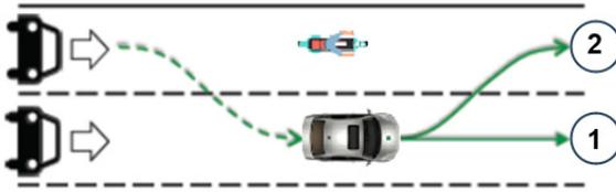
**Figure 1:** Two options for overtaking a motorcycle in the left-hand traffic system.
