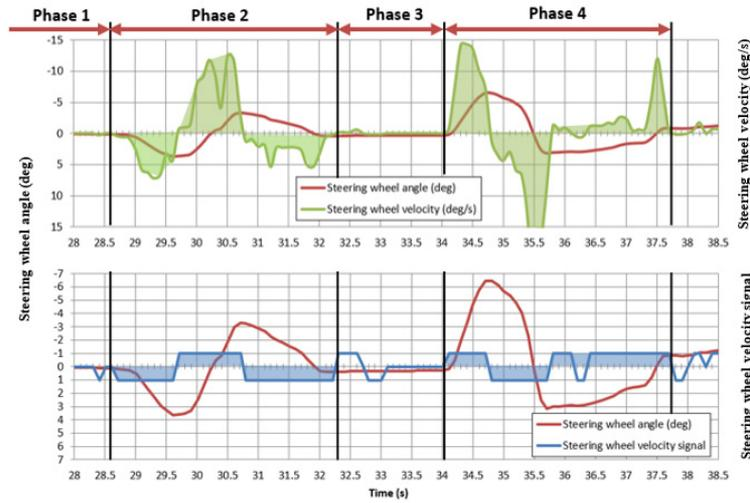
**Figure 6:** Time course of the steering wheel angle and steering wheel velocity when performing overtaking maneuver: raw data (above) and after signal conversion (below).
