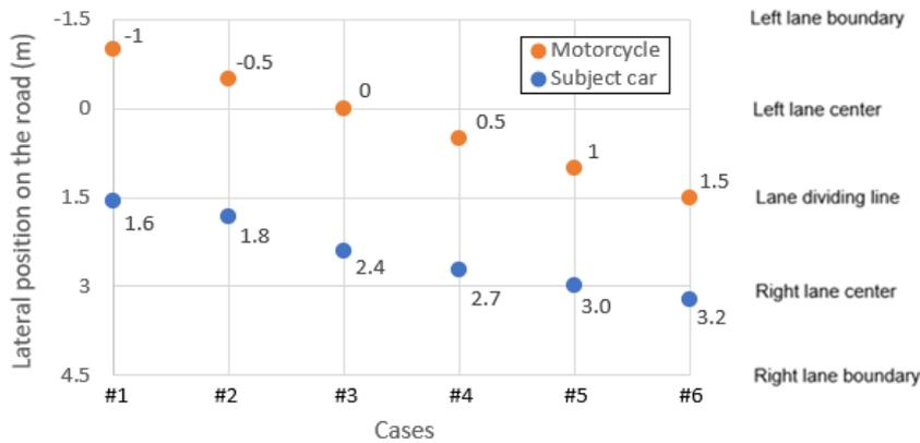
**Figure 9:** Average lateral positions of subject car and motorcycle in phase 3 in different conditions.
