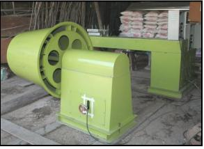
Figure 3: Automatic fiberglass winding machine [3]
