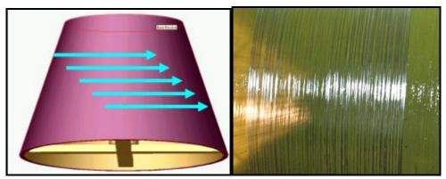
Figure 5a: Schematic of close winding format and Figure 5b: Physical close winding format
