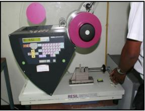
Figure 8: Izod impact test set-up
