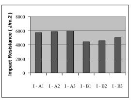
**Figure 11:** Impact resistance of sample cut along the fiber winding direction
