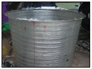
**Figure 4:** Sample of fiberglass tank from automatic fiberglass winding machine
