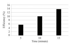
**Figure 12**: The efficiency of pressing palm at a speed of 155 rpm after dried with hot air.
