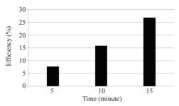
**Figure 8**: The efficiency of pressing palm at a speed of 133 rpm before dried with hot air.
