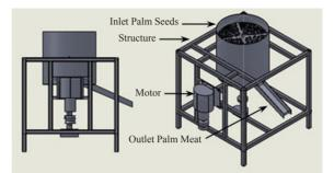
Figure 1: Palm seed separating machine plan.
