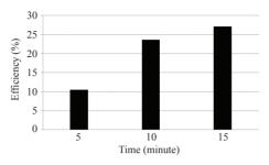
**Figure 10**: The efficiency of pressing palm at a speed of 110 rpm after dried with hot air.
