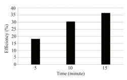
**Figure 9**: The efficiency of pressing palm at a speed of 155 rpm before dried with hot air.
