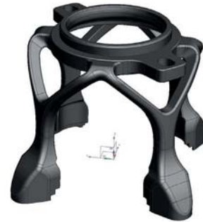
Figure 5: Load bearing metal framework of pump housing developed using topology optimization method.
