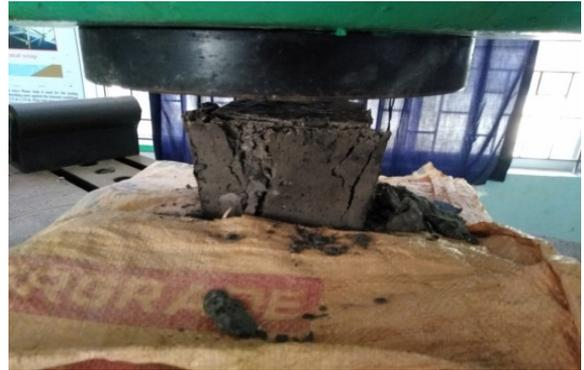
**Figure 1:** Compressive strength of the LCGPC cubical specimens.
