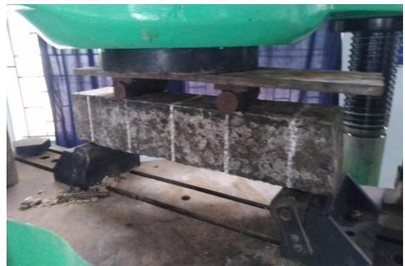
**Figure 2:** Flexural strength of LCGPC prism specimens.
