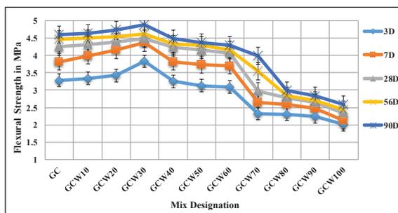
Figure 7: Flexural strength of LCGPC.
