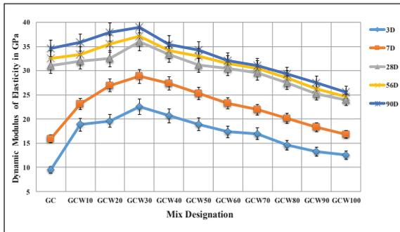
**Figure 8:** Dynamic elastic modulus of LCGPC.
