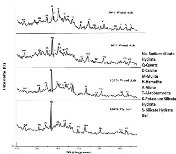
**Figure 10:** XRD Analysis of LCGPC Mixes.
