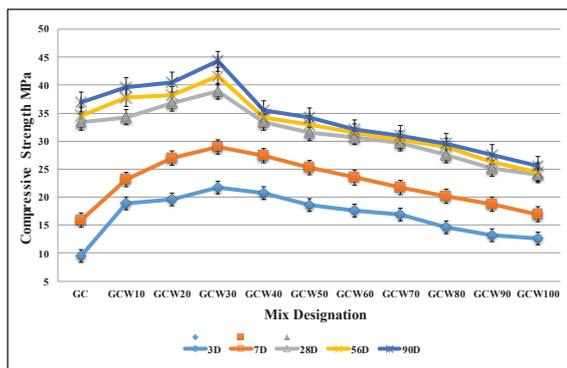
Figure 6: Compressive strength of LCGPC.
