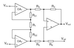
Figure 1: Instrumentation amplifiers circuit [21].
