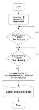
**Figure 4**: Programing process for watermelon sorting operation.
