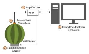
**Figure 5**: Principle operation of the sorting machine [10].
