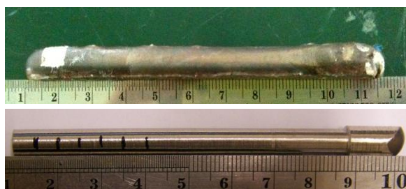
Figure 1: Weld metal specimens; (top) from simulated, (bottom) after prepare cylindrical shape.
