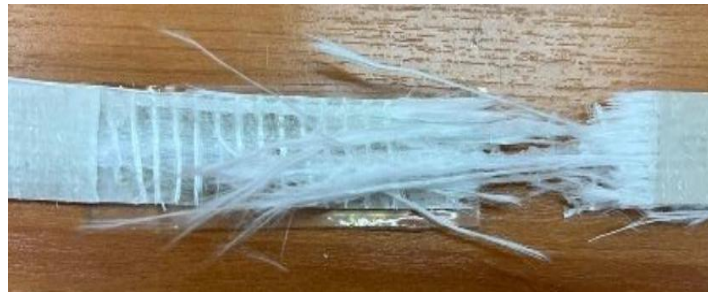
Figure 2: Failure patterns of LC-GFRP testing.
