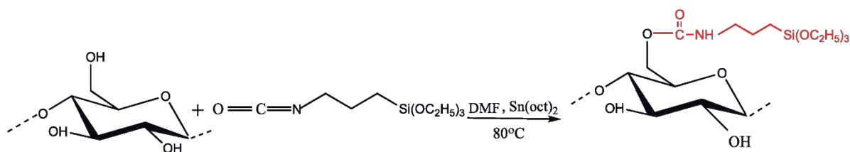
Figure 7: Reaction scheme for CNCs surface modification using IPTS. Reproduced from [25].
