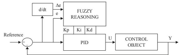
Figure 4: The adaptive Fuzzy-PID controller schematic [1].
