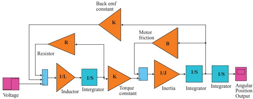
Figure 2: DC motor model in Simulink.
