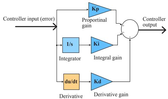
Figure 3: Schematic of the PID controller.
