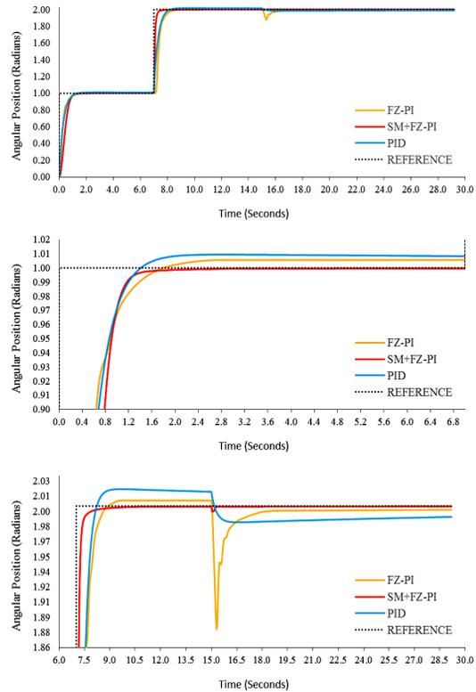
Figure 9: DC motor position response during normal operation.
