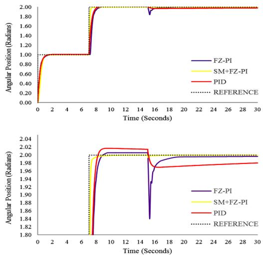
Figure 11: DC motor position response to torque load during 50 percent increase in resistance.
