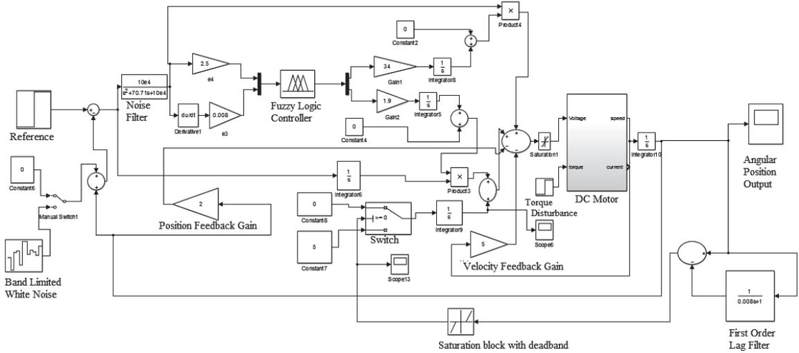
Figure 5: First order lag adaptive sliding mode controller architecture modelled in SIMULINK.
