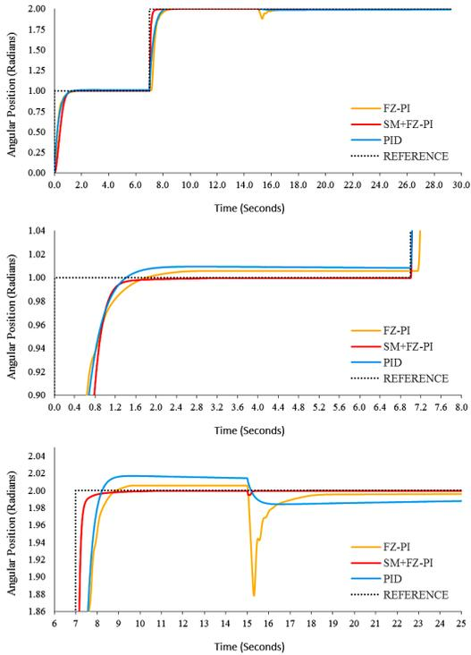
Figure 10: DC motor position response during 50 percent increase in motor inertia.
