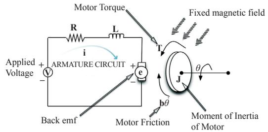
Figure 1: A schematic diagram of a DC motor [9].
