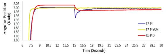
Figure 12: Effect of feedback loop random white noise.
