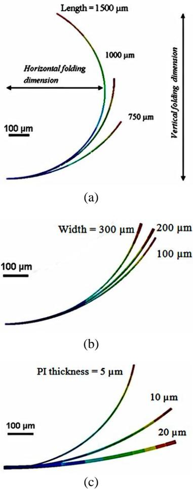
**Figure 3:** Folding shapes for various beams; (a) various lengths with the fixed width of 100  $\mu\text{m}$  and polyimide thickness of 5  $\mu\text{m}$ , (b) various widths with the fixed length of 750  $\mu\text{m}$  and polyimide thickness of 5  $\mu\text{m}$ , (c) various polyimide thicknesses with the fixed length of 750  $\mu\text{m}$  and width of 300  $\mu\text{m}$  (all cases have NiTi thickness equal to 1  $\mu\text{m}$ ).
