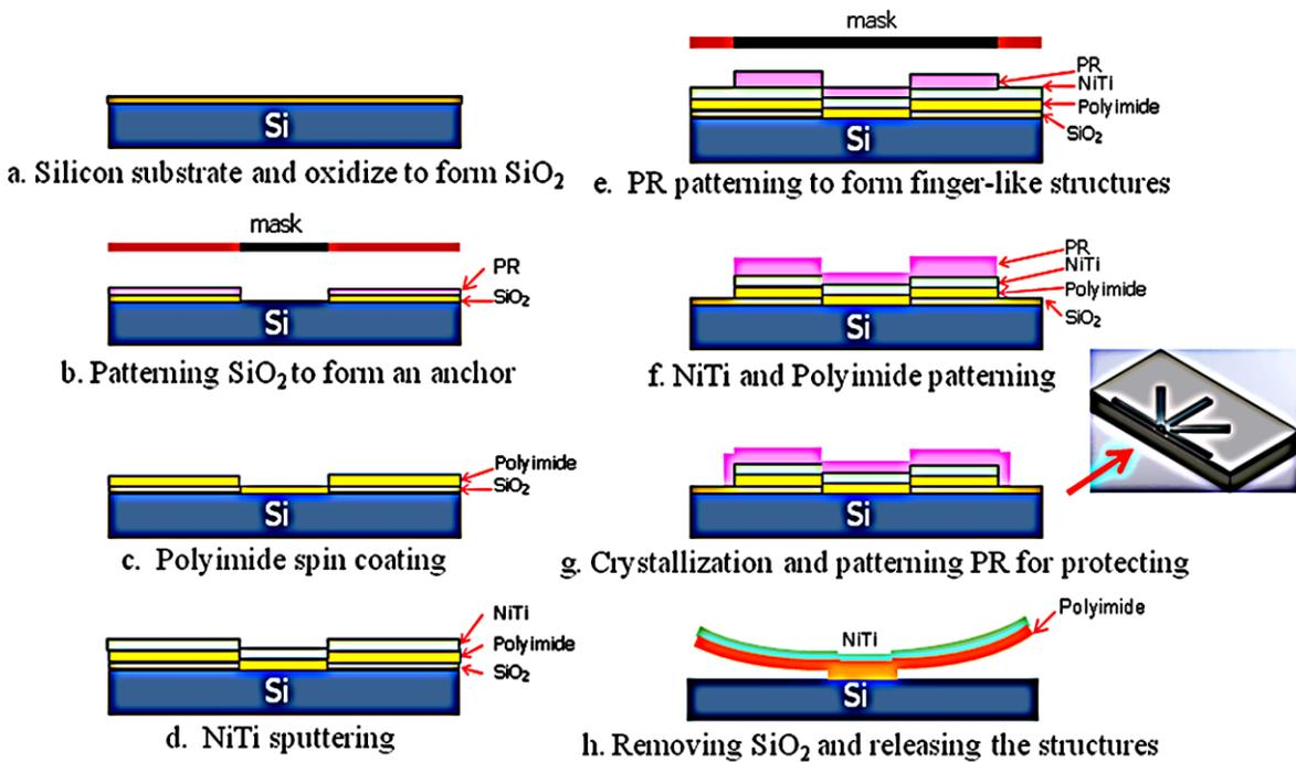
**Figure 6:** Micro fabrication processes for the proposed micro-gripper.
