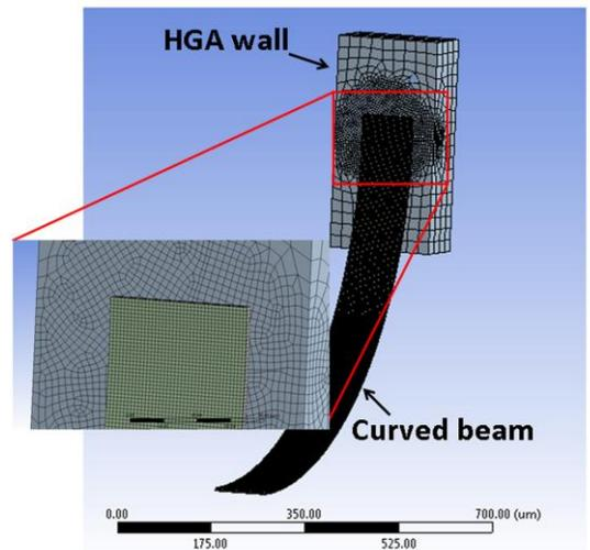
**Figure 5:** Simulation domain of contact force between micro-actuator and HGA.
