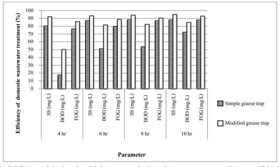
**Fig. 3.** Efficiency of simple and modified grease traps for domestic wastewater treatment (flow rate of 2 L/min, HRT varied between 4-10 hrs).
