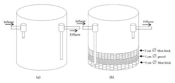
Fig. 1. Schematic diagrams of (a) simple grease trap and (b) modified grease trap of Mon brick and gravel.
