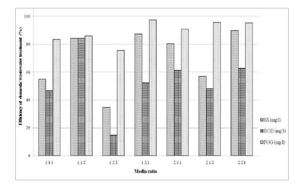
Fig. 2. Effect of media ratios on efficiency of modified grease trap treating domestic wastewater.
