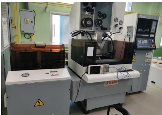
Fig. 2 The JSEDM series W-B430 machine
