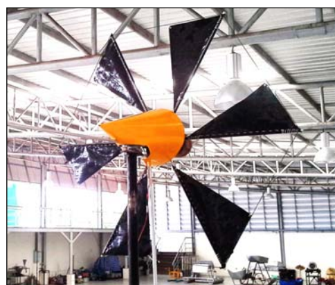
Fig.2 Downwind Thai sail windmill [3]
