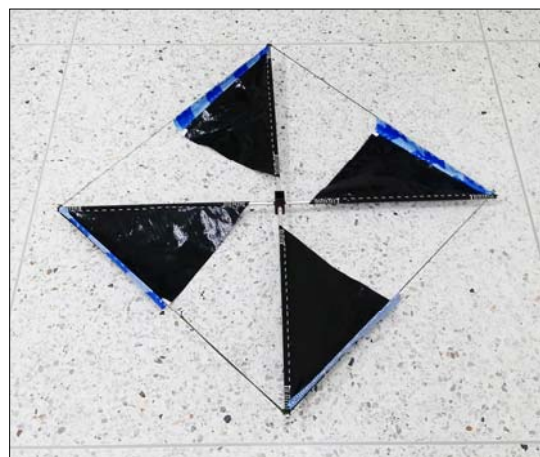
Fig.7 The 4-blade rotor by using the technique of closing the blade tip (Closed-tip DTSW)
