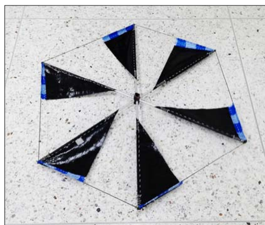
Fig.8 The 6-blade rotor by using the technique of closing the blade tip (Closed-tip DTSW)
