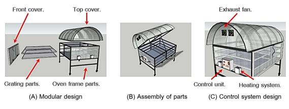
Fig. 1 Design characteristics of the electric oven with solar energy
