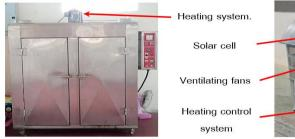
Fig. 2 The former three-phase electric oven
