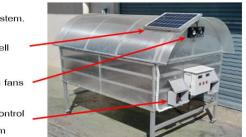
Fig. 3 Electric oven with solar energy
