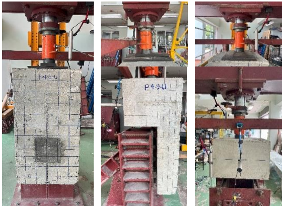
Figure 6: Push-off test set-up (Front, Side and Back View) and Installation of load cells and LVDTs.
