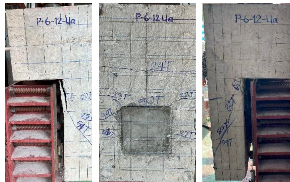
Figure 7: Crack patterns of the specimen P-6-12-Ua from the left-side, front-, and right-side-view.
