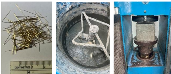
Figure 5: Steel fiber; mixing of UHPC; and cubic compressive strength test.
