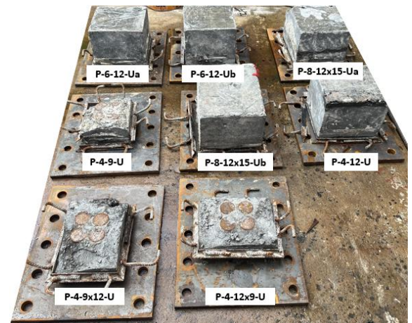
Figure 11: Internal section and shear cut failure of UHPC shear pocket.
