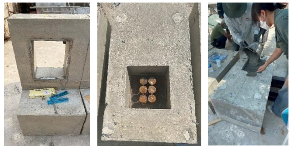
Figure 4: Strain gauges installed to the angle confinement; Studs arranged in the shear pocket; and UHPC filled in the pocket.
