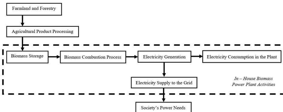
**Figure 3:** A general concept of biomass-based power plant operations.
