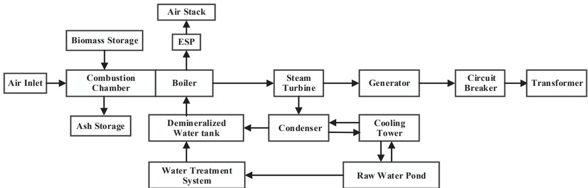
Figure 5: The electricity generation process in the case study.
